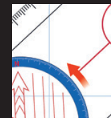
Rotate the compass housing to compensate for magnetic variation
