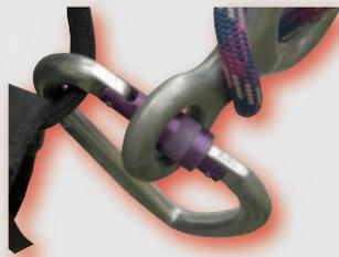
**3.** If the rope is then weighted again the figure of eight can both load the karabiner axially and apply leverage to the gate. The size of loads generated in abseiling and belaying when coupled with this leverage can be sufficient to damage the sleeve of the screwgate.
