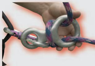
Tests on one particular type of karabiner showed that loads of just 1kN would be enough to damage the gate and force the karabiner open. Depending on
