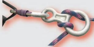
**2.** If tension is not maintained between the figure of eight and the screwgate, there is a tendency for the figure of eight to turn over and take up an abnormal configuration in relation to the karabiner.
