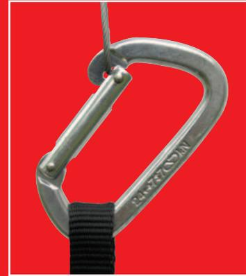
If fallen on when clipped like this, the karabiner will be loaded gate open and could fail completely with a fall of only a few feet.
