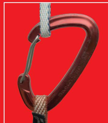
The new narrow spectra slings can compound this problem. Here at least the gate is completely closed, but this may not always be the case.
