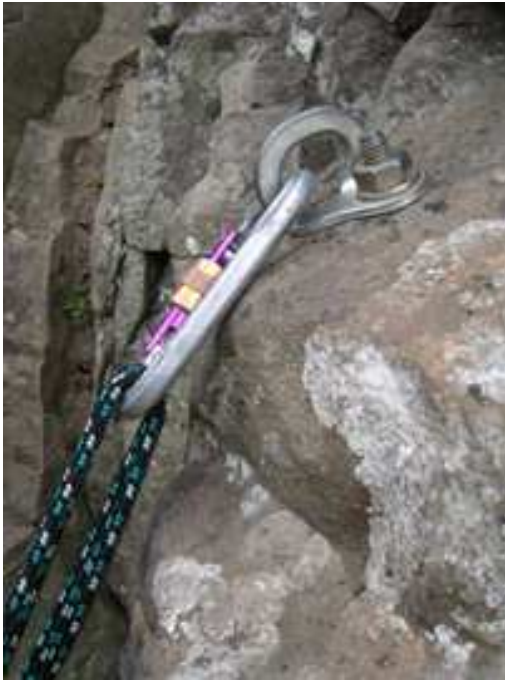
Leverage could damage the karabiner; also the bolt is quite close to an edge.
