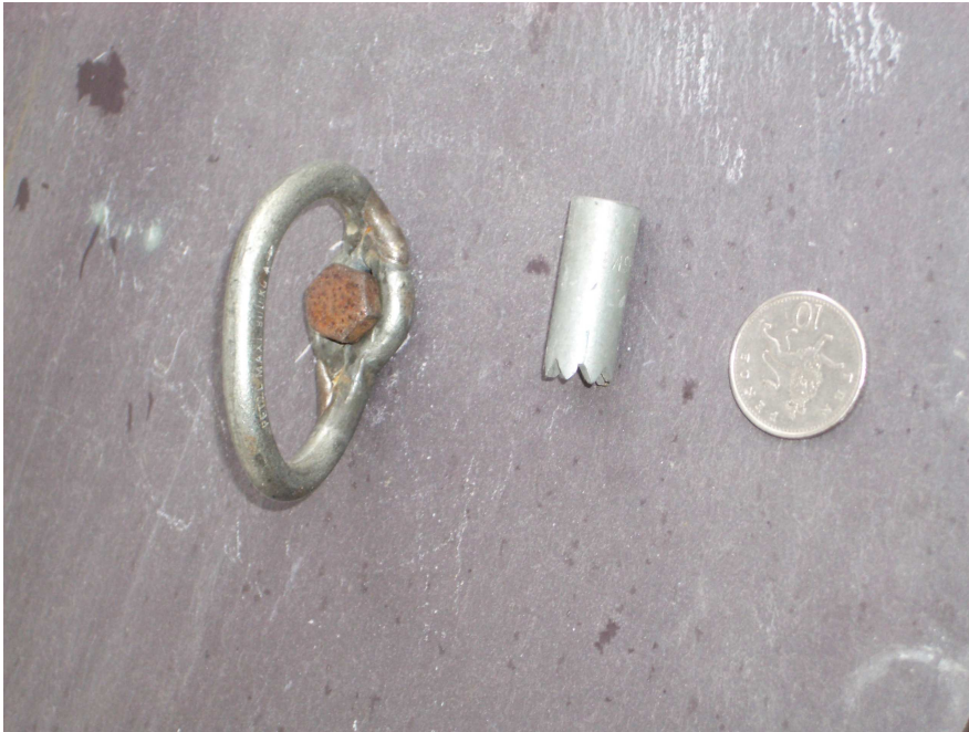
Old bolts may provide only an illusion of safety. When new this bolt was rated for aid only.
