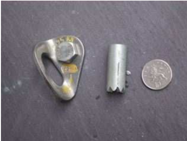
8mm Self Drill Bolt or Spit. Note the depth of the fixing!
