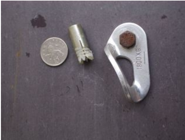
Petzl 8mm self-drilling anchor.
