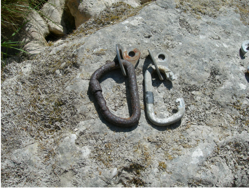
Alloy and steel krabs quickly become useless.
