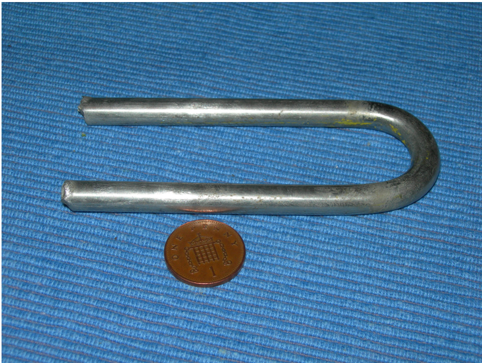
This early version of a staple pulled out at a very low load. Without notching or filing there was nothing for the glue to key onto.
