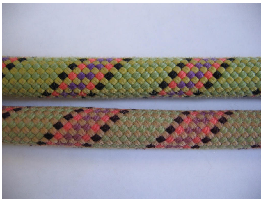
Comparison of two areas of the rope sheath, showing discolouration.
