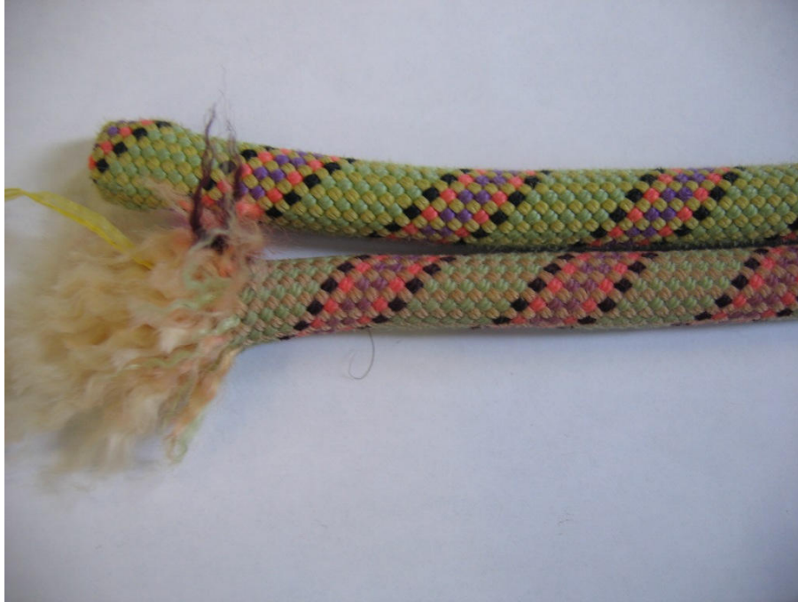
Discolouration around the area of the break.
