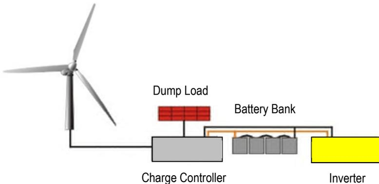
Diagram of an off-grid wind generation system with a dump load. In huts that have mains electricity the power can be fed into the existing wiring circuits and excess power can be exported to the grid and sold to energy suppliers.
