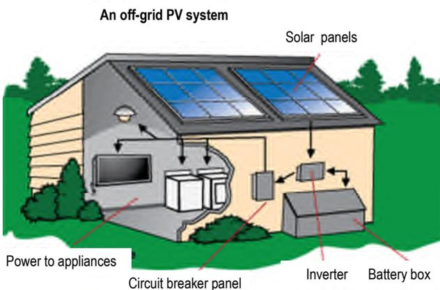
PV systems generate electricity which can be used to power lighting and, with larger capacity systems, electrical appliances such as microwave cookers. An off-grid system is shown in the diagram. DC current from storage batteries is converted to AC (240 v) by an inverter. PV panels are usually roof mounted although they can also be mounted on the ground. If a hut has a mains electricity supply then surplus power can be sold to the grid.
