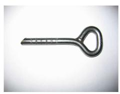
A small number of these are available. Compared to the other resin bolts, they need a much smaller hole, which saves time and battery power. The manufacturer recommends using Hilti HIT HY150 resin, which isn't cheap and needs a special dispenser. The weld means that they aren't suitable for sea cliff use, but they would be ideal for inland crags where rock quality isn't great.
