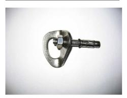
If you've sport climbed abroad, you've probably seen a few of these before. Quick and easy to place, they are limited to use on hard/medium rock. Although they are made from AISI316 for corrosion resistance, the basic design is not really ideal for use on sea cliffs. If used to make up belays, maillons will have to be added.
