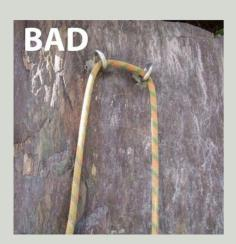
To address the problem the BMC and The NWBF (North Wales Bolt Fund) have recently purchased 300 marine grade stainless steel maillons and 300 marine grade stainless steel certified welded rings - this is sufficient for 150 lower-offs and should be sufficient to sort most of the popular routes on upper and Lower Pen Trwyn.
