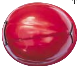
The HB Astral after a test impact: Note the striations
