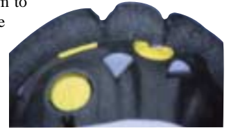
A cut away of the Petzl Meteor following a penetration test.
