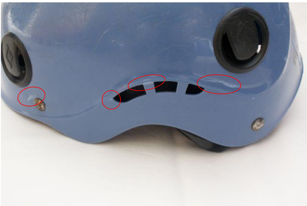
Figure 4: Helmet LHS with deformation marks circled
