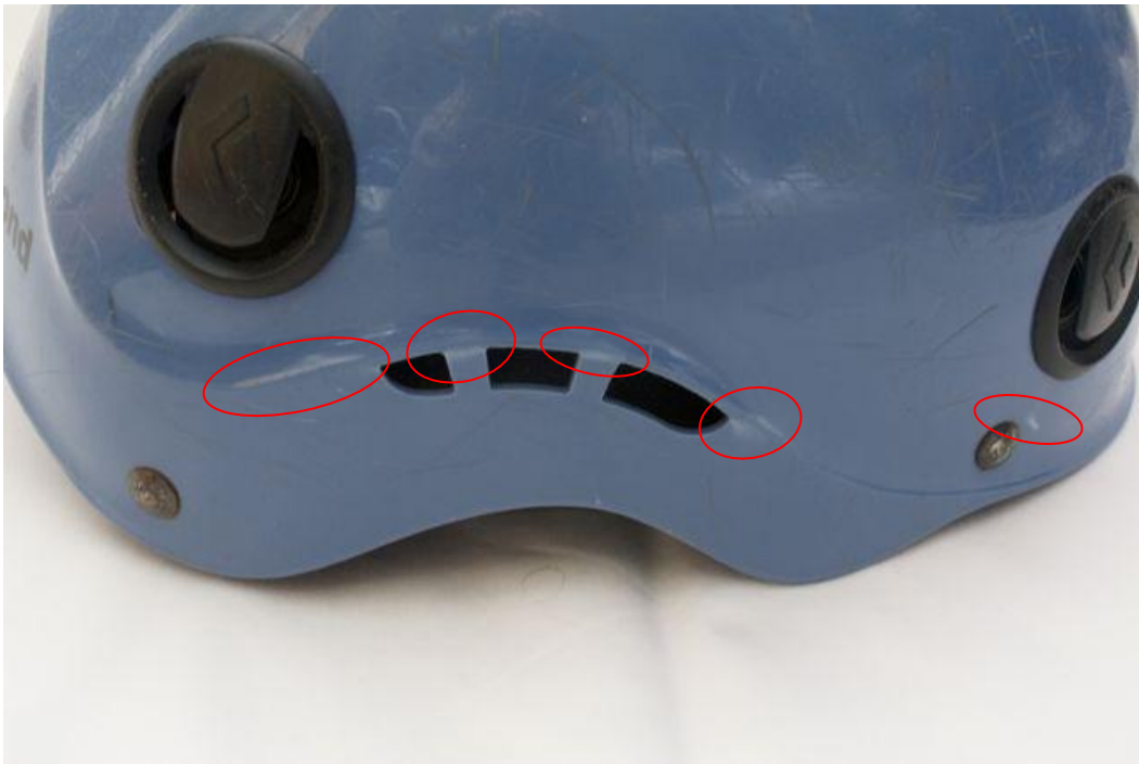
Figure 3: Helmet RHS with deformation marks circled
