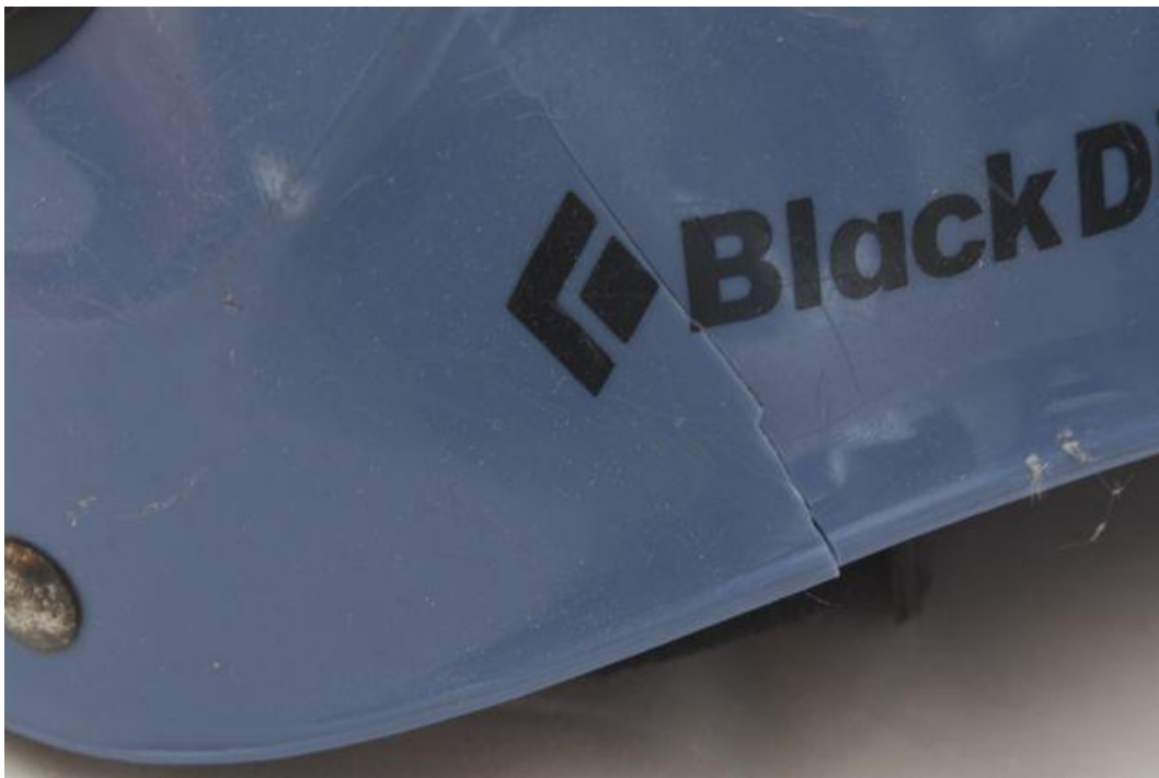
Figure 2: Crack on rear rim
