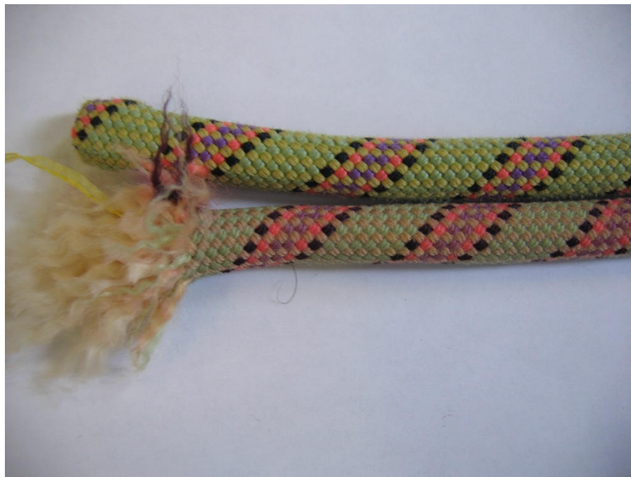
Discolouration around the area of the break.
