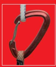
The new narrow spectra slings can compound this problem. Here at least the gate is completely closed, but this may not always be the case.
