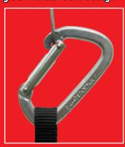
If fallen on when clipped like this, the karabiner will be loaded gate open and could fail completely with a fall of only a few feet.
