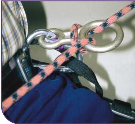
Figure 1.3 A figure-of-8 forcing open a screwgate karabiner.
