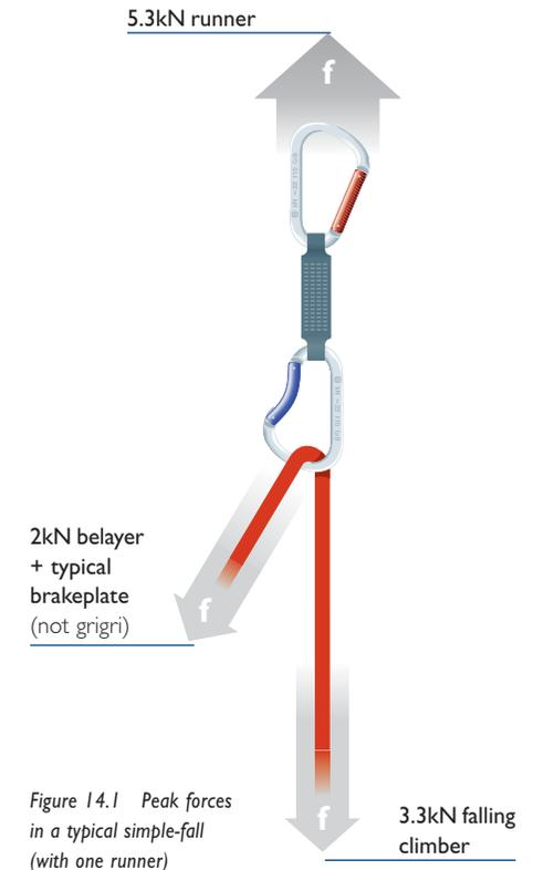
Figure 14.1 Peak forces in a typical simple-fall (with one runner)
