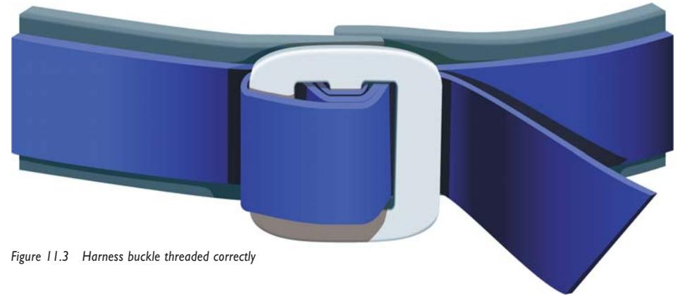
Figure 11.3 Harness buckle threaded correctly
