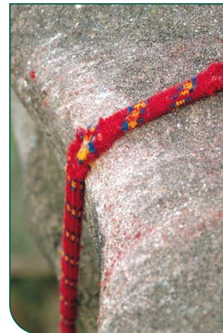
Figure 10.3 Serious damage to a rope in use
