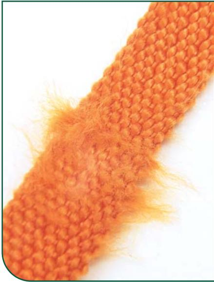
Figure 11.4 Frayed/damaged webbing
