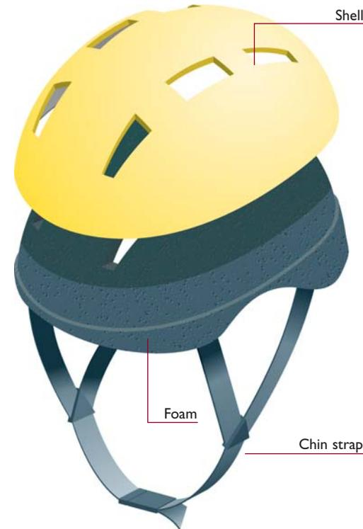
Figure 9.3 Expanded polymer foam helmet
