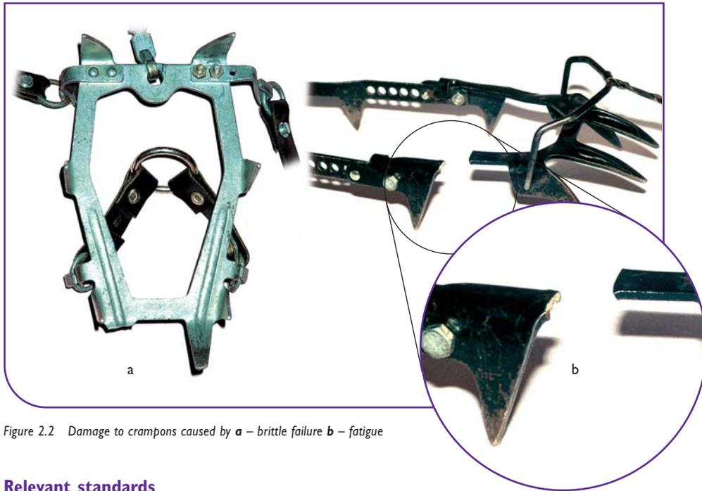
Figure 2.2 Damage to crampons caused by **a** – brittle failure **b** – fatigue
