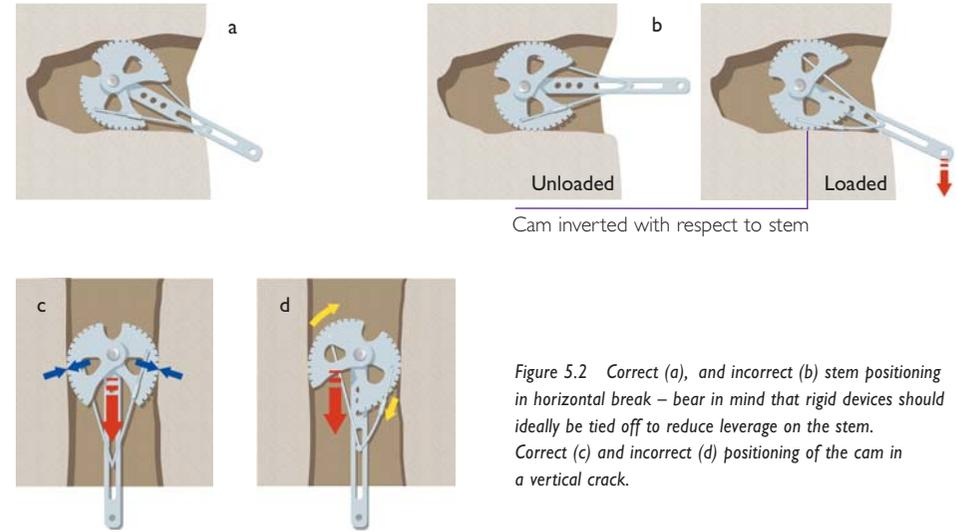
Figure 5.2 Correct (a), and incorrect (b) stem positioning in horizontal break – bear in mind that rigid devices should ideally be tied off to reduce leverage on the stem. Correct (c) and incorrect (d) positioning of the cam in a vertical crack.
