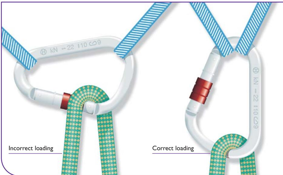
Figure 1.4 Three-way loading of screwgate karabiner
