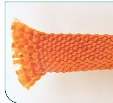
Figure 12.2 Cut, damaged yarn
